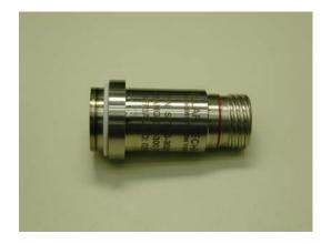
2) Insert Transducer into adapter until seated.
